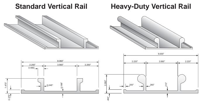
Cross Section of Standard Vertical Rail Cross Section of Heavy-Duty Vertical Rail
