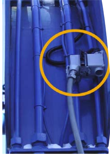
Fig.5 Quick disconnect plug onto the stick boom
