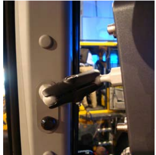
Fig.11 Komatsu -7 series cabin pillar has M10 female thread
