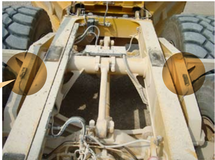
Fig.1 ADT walking beam with Load Links on it
