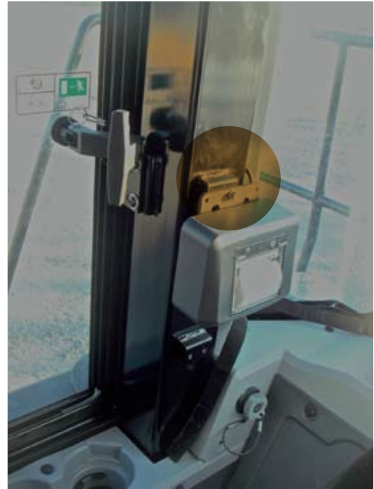
Fig.4 vprint fixed separately on the rear right pillar of a cabin using the standard plate to attach the printer underneath the Device
