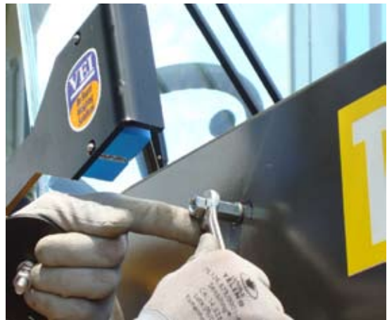
Fig.12 Installing Weighing Zone reference hexagon
