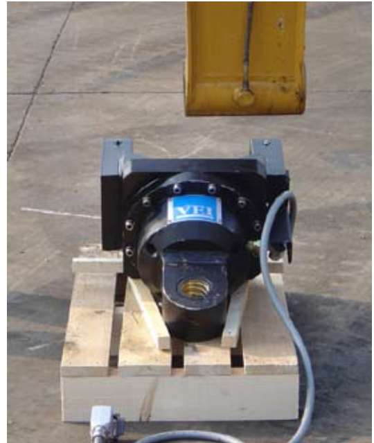
Fig.3 Sliding Stick boom into the GR2 upper plate
