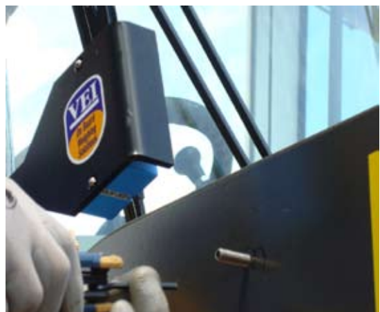
Fig.11 Installing Weighing Zone reference headless screw
