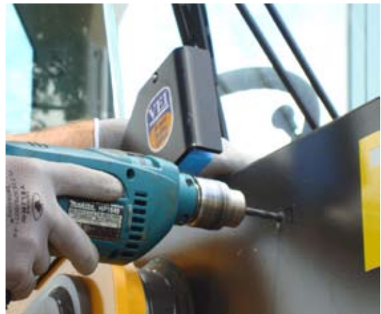
Fig.9 Drilling Weighing Zone reference fixing point
