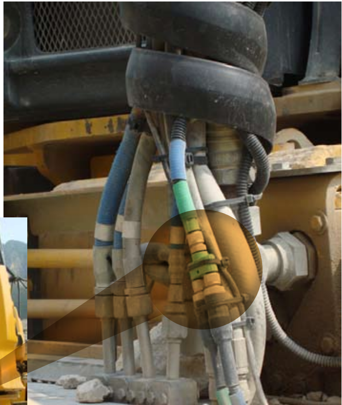
Fig.2 Load Links Y splice junction
