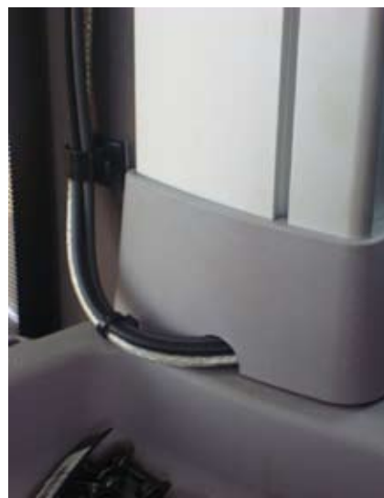
Fig.4 Harness fixed onto the pillar
