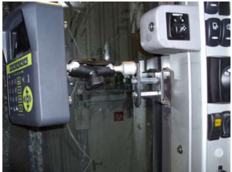
Fig.19 Volvo G series with mirror command. The Device bracket can be fixed on 2 exagon in order to place the Device out of the rear view mirror command. As an alternative the mirror command can be slid up or down.
