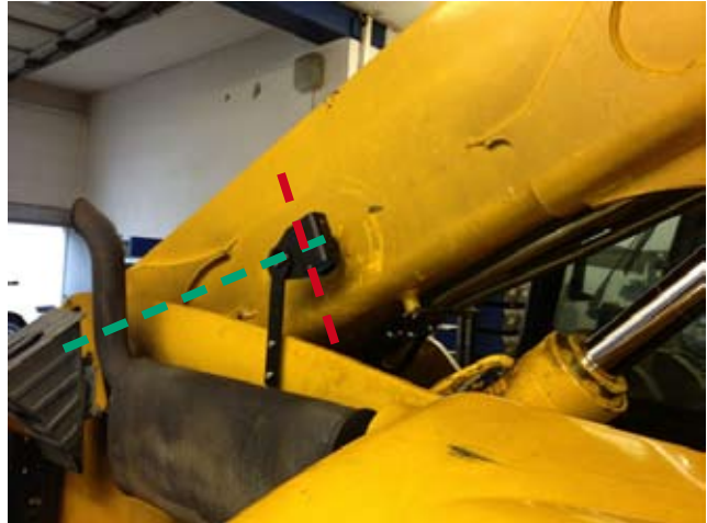
Fig. 3 Weighing Zone Reference moving position through the Weighing Zone Sensor
