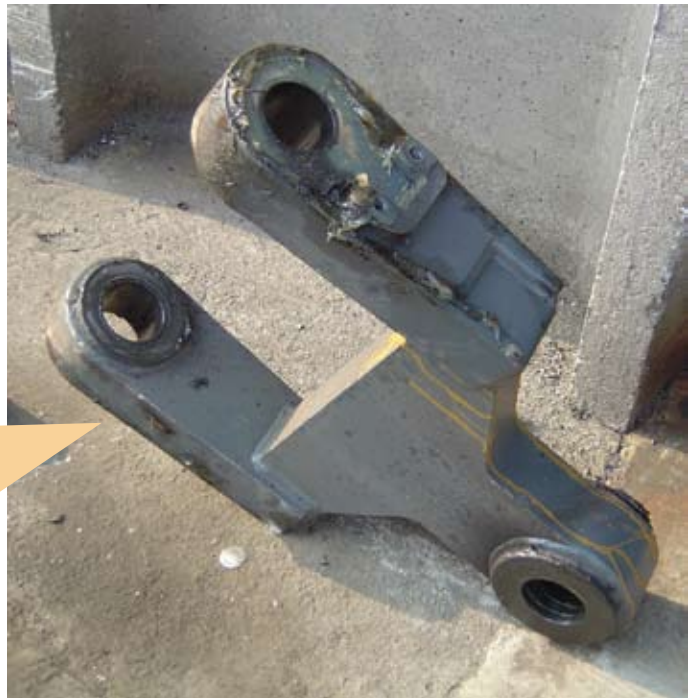
Fig.2 Original Yoke uninstalled
