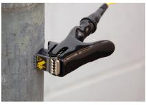
Good contact between the cable lead and the target conductor lowers the resistance of the circuit and produces a stronger tracing signal.
