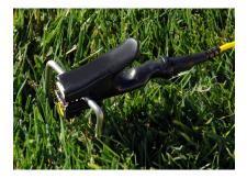
Instead of using the provided grounding stake, the lead clip can be attached to other objects such as a shovel blade or a metal rod sunk into the earth. Using larger grounding objects may improve grounding by increasing the surface area in contact with the earth.
