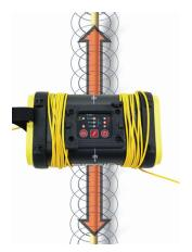
Press the Power key () to power on the ST-305/R. Press the Inductive Mode key () to toggle the ST-305/R between Direct Connect Mode and Inductive Mode.
